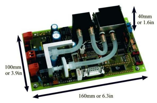
The CarbonOxy is a unique device for measuring CO2 and O2 on a Euro Printed Circuit Board (PCB). Carbon Dioxide is measured using the dual wavelength technique (NDIR - Non-Dispersive Infra Red) while Oxygen is measured using Zirconium Oxide. This combination ensures a quick response time along with elimination of interference from other gases.
